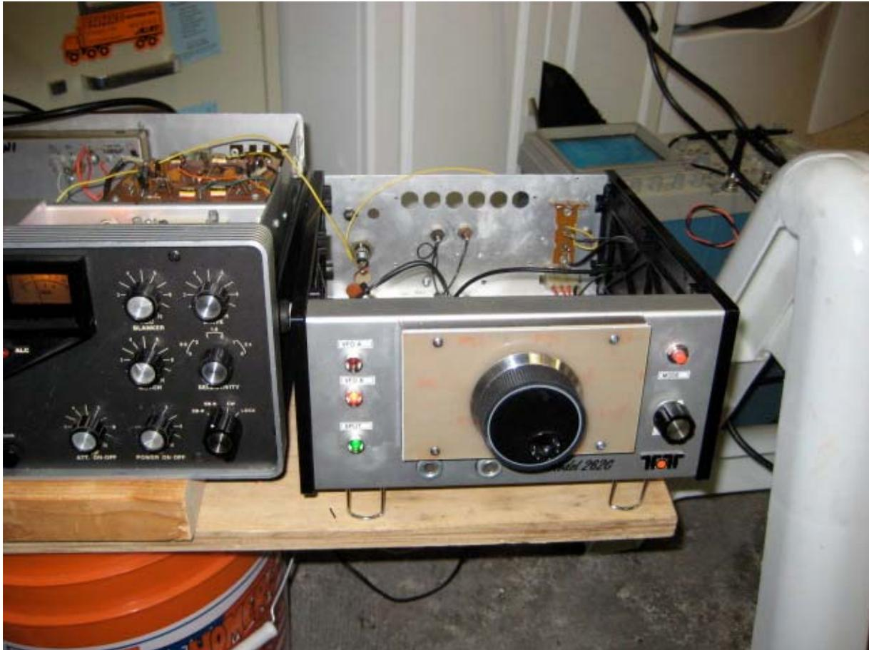
First some baseline information about the stock Omni D which is essentially a single conversion radio with a 9.0 MHz IF. On all stock bands except 20M, the 5.0 MHz PTO signal is heterodyned with various crystal frequencies to provide the proper injection frequencies. You will note that the Omni D as well as other Ten Tec Radios define their SSB operation as normal and opposite versus USB or LSB.
