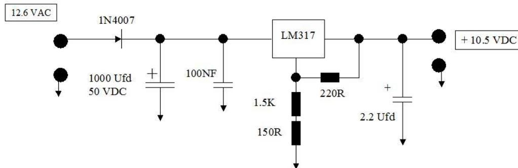
The 220 Ohm and 1650 Ohm Resistances set the 10.5 VDC level
