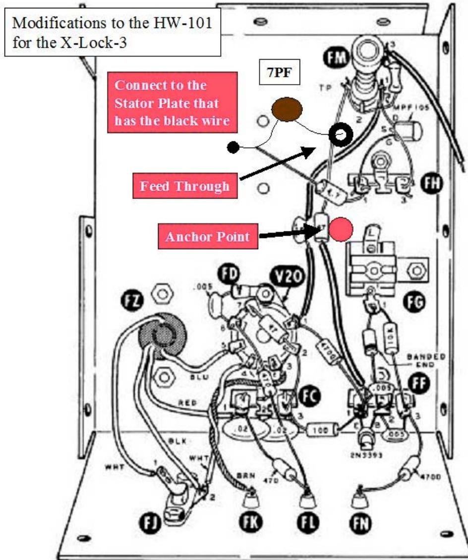
Two pass through devices are installed in the HW-101 VFO Case. One is modified to act as a “feed through” type and the other is an anchor point that is used to make connections on the top side of the case. The 100K resistor is connected to these two points on the outside of the VFO. The 7PF cap is connected from the Feed Through to the Tank.
