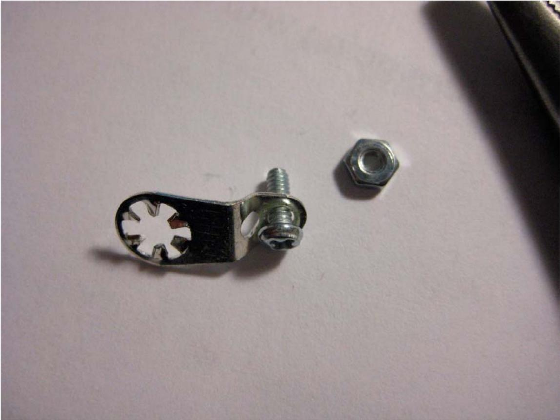
The #4 solder lug is bent into a “Z” shape using a pair of needle nose pliers. For attachment to the PC board, 1/4 inch long 2-56 screws are used. This forms a very stout mechanical connection.
