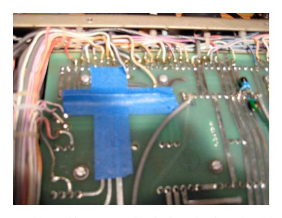
I used 3M masking tape to provide a barrier so the PC Board would not short to the Motherboard traces.
