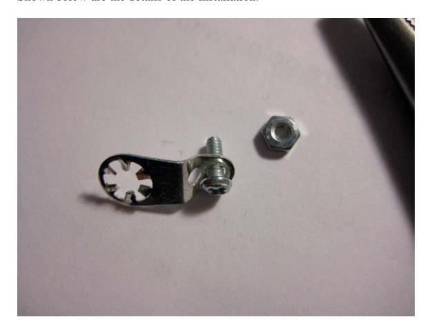
The #4 solder lug is bent into a "Z" shape using a pair of needle nose pliers. For attachment to the PC board, ¼ inch long 2-56 screws are used. This forms a very stout mechanical connection.
